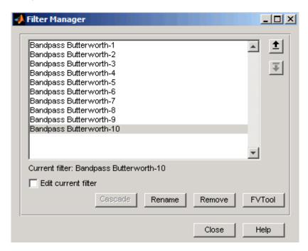
**2** Press Ctrl+click on each filter name to select all the filters, and then click **FVTool**. FVTool opens with the filter responses overlaid for easy comparison. (If you want to view a single filter in FVTool, click the **Full**
